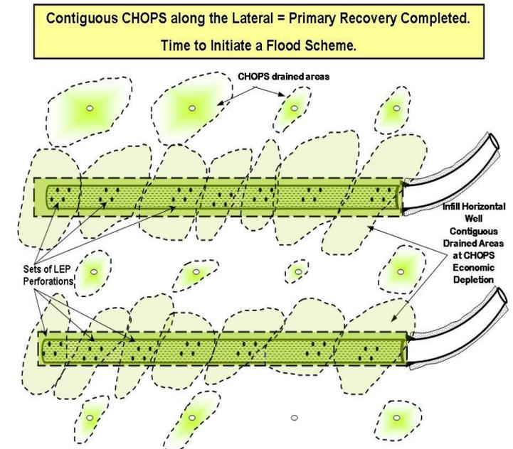
**Figure 2.** The expanded drained areas along the horizontal well created by sequential Limited Entry Perforations (LEP) are conceptual overlays.
