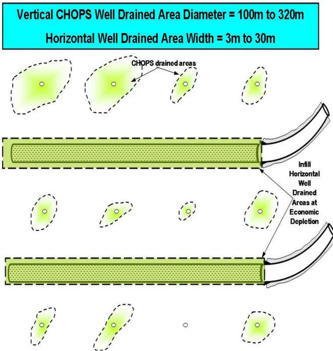
**Figure 1.** Illustrates drained areas surrounding vertical CHOPS wells identified by 3D seismic. Infill horizontal wells with pre-CHOPS drained areas are conceptual overlays.
