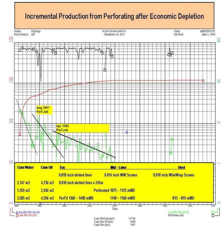
**Figure 3.** Description of the Horizontal well slotted liner segments, sequential perforation intervals, and production associated with each.
