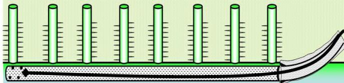
**Figure 4.** On a new well the cost estimate follows the sequence: 1. Produce the entire slotted liner to economic depletion using a jet pump landed at the first slots below the Heel. 2. First re-completion follows at the Toe. 3 Subsequent re-completions move uphole to the Heel.
